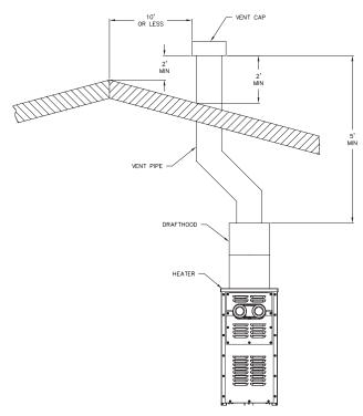
Figure 7. Vent Piping Requirements.
